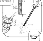
The oil level is correct when it is at the **full** mark on the dipstick. **DO NOT OVERFILL.**
